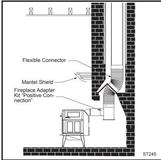
**Fig. 8** In this installation, the chimney connector enters the firepalce opening and then connects to the chimney.
